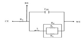
Figure (7): The equivalent circuit model used to fit the experimental data.
