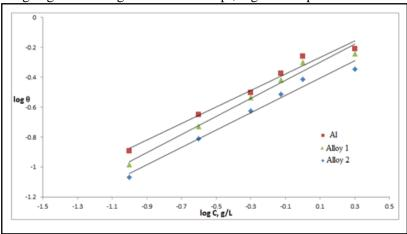
**Figure (3):** The relation between log ( $\theta$ ) and log C, g/L for aluminum, alloy I and alloy II electrode in 0.1 M NaOH solution and different concentrations of methyl cellulose.
