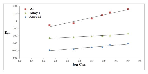
Figure (10): The relation between the pitting potential  $(E_{pit})$  and  $\log C_{inh}$
