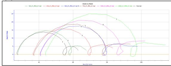
Figure (6): Nyquist plots recorded for alloy II electrode in 0.1 M NaOH solution and different concentrations of methyl cellulose at 30°C.
