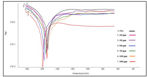
Figure (2): Anodic and cathodic polarization curves for aluminum electrode in 0.1 M NaOH solution and different concentrations of methyl cellulose at scan rate of 10 mV/sec
