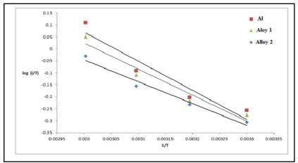
**Figure (5):** Plots of log (i/T) versus 1/T for aluminum, alloy I and alloy II electrodes in 0.1 M NaOH solution + 2000 ppm of methyl cellulose.
