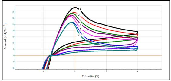
Figure (8): Cyclic voltammetry curves for aluminum electrode in 0.1 M NaOH solution and different concentrations of methyl cellulose at scan rate of 1 V/sec.
