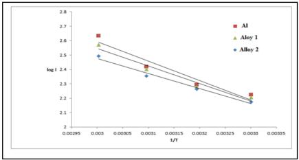
**Figure (4):** Arrhenius plot for aluminum, alloy I and alloy II electrodes in 0.1 M NaOH solution + 2000 ppm of methyl cellulose.
